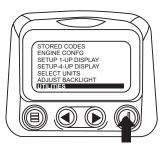
4. Touch "Select" to enter the "Gage Data" display. When "Gage Data" is selected the PowerView will communicate with the analog gages at a fixed rate of 38.4k Band, 8 data bits, no parity check, 1 stop bits, half duplex.
